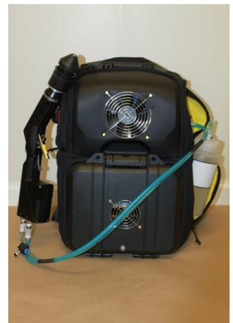
Patented Air-atomizing Induction-charging nozzle
