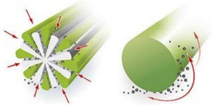
The ICS Greenspeed<sup>®</sup> microfiber is split so that an elaborate system of hollow tubes is created. These hollow tubes have two major advantages:
