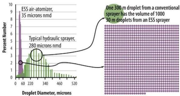
Electrostatic spraying provides superior spray coverage by more effectively dispensing solutions than conventional sprayers. Tests have demonstrated up to 10 times better coverage resulting in reduced manpower costs and reducing the threat of disease-causing microorganisms.
