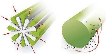
The ICS Greenspeed<sup>®</sup> microfiber is split so that an elaborate system of hollow tubes is created. These hollow tubes have two major advantages:
