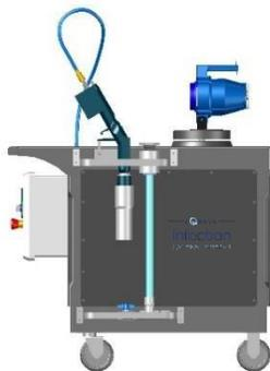
This induction charging results in spray droplets that have a force of attraction of 75 times that of gravity. This means droplets will reverse direction and move upwards, against gravity, to coat hidden surfaces, and wrap around objects resulting in complete, even coverage of the target.
