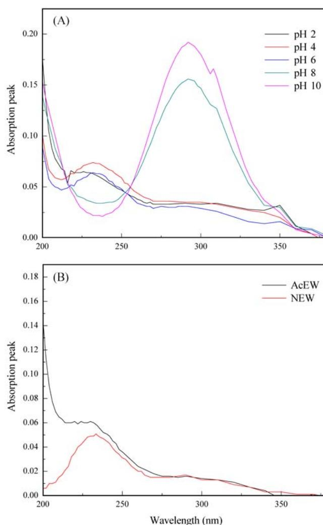
**Fig. 3. Ultraviolet (UV) spectroscopy of the ClO<sup>-</sup> in solution. (A), serial pH values of the NaClO solution; (B), in AcEW and NEW solutions**
