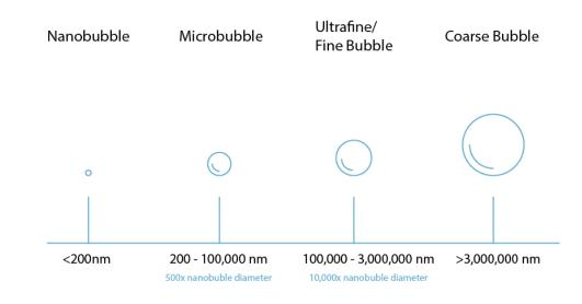
The Aquaox Nanobubble generation method consistently produces high density solutions of optimally sized nanobubbles, averaging 100 nm in diameter and ranging between 50 and 100 nm.
